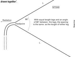
My version of the antenna, as described in this article, slopes down towards the open ends of the V, which further lowers the radiation angles on the higher frequency bands. With a horizontal 'V', the vertical angle of radiation is quite low, at 31° when the leg length is only one wavelength.
